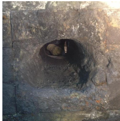
Taphole after 21,250 metric tons of hot metal
